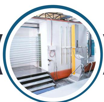
Kenan Metal has a production capacity of 18,000 tons with a 12-meter electrostatic paint line. It carries out painting operations with a power and free z-type electrostatic paint booth with a capacity of 12,000 tons and a tunnel-type electrostatic paint line with a capacity of 7,200 tons.
